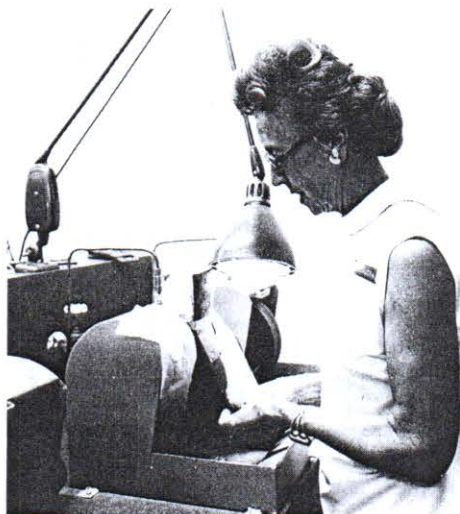
A good idea developed here is the splashless water feed. Even if it is splashless, this gem cutter isn't going to let any spray get out of the water guard.
